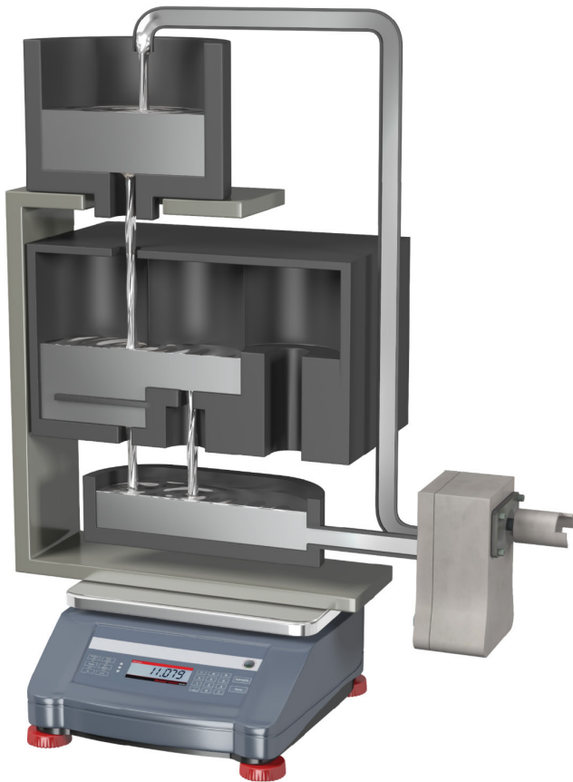
Extended Data Figure 4 | Experimental set-up of the calibration of the visual flow meter. The weight-based flow meter was positioned above the visual flow meter and the pump speed was adjusted until the desired flow (for example, through only two outlets or through three outlets) was achieved. Under these conditions, flow was monitored from both flow meters so that the quantitative information from the weight-based flow meter could be related to the qualitative information from the visual flow meter.
