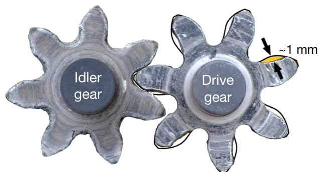
Figure 5 | Wear on Shapal gear teeth after 72 h of continuous pumping. The black outline behind the drive gear indicates the original shape. The yellow shading and arrows highlight the width loss of about 1 mm.
